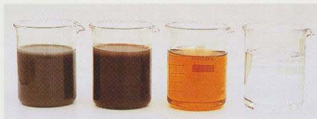
Raw water Activated sludge MF treated water RO treated water
